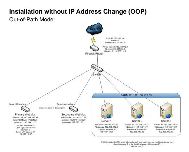
The above diagram is an example about how to configure the WebMux<sup>™</sup> in outof-path mode without changing the IP addresses of the web servers and other servers that already exist on the network. This is particularly helpful when the changing of an existing network of servers causes problems.
