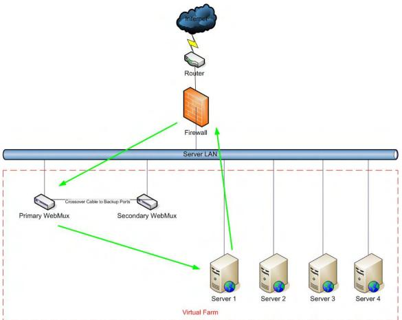
In most situations, the incoming traffic is in small requests, and return traffic from servers back to clients is large amount of data, pictures, or documents. Using out-of-path mode will allow up to 100 times more traffic to be handled by the
