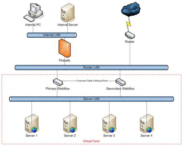
The main purpose of the WebMux<sup>TM</sup> is to balance the traffic among multiple web or other servers. The diagram above shows a NAT installation with two WebMuxes. In this configuration, one WebMux<sup>TM</sup> is serving as the primary, and the other is serving as the secondary, or backup, providing a fault tolerant solution.
